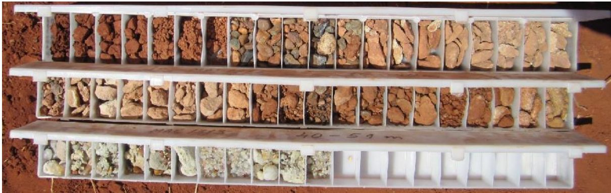
Figure 8 – Drill chip samples from Manyingee aircore hole MAC006 showing orange Quaternary clayey sand and gravels to 12m; oxidised glauconitic sandy claystone (Tertiary) at 12-37m; Yarraloola conglomerate at 37-47m; weathered granitic basement 47-51m. The prospective Birdrong sandstone is absent.
